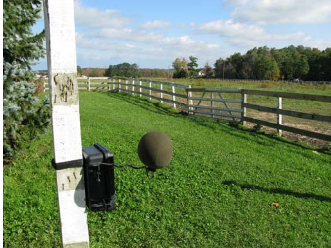
Figure 4.3.3.2 Typical Integrating Sound Monitor with 7" Weather-treated Windscreen
